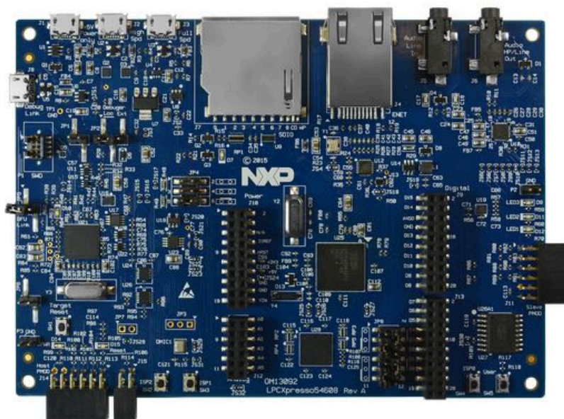
Figure 2. LPCXpresso development board (LPCXpresso54608)
